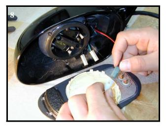
Cut a slot in the foam disc just large enough to accommodate the anti-rotation prongs on the motor adaptor (on the *Signal*® mirror). Place the foam disc on the back of the *Signal*® mirror. If your mirrors have the heater option, connect the heater mirrors at this time. Connect the *Signal*<sup>®</sup> mirror mating connector to the *Signal*<sup>®</sup> mirror wire harness.
